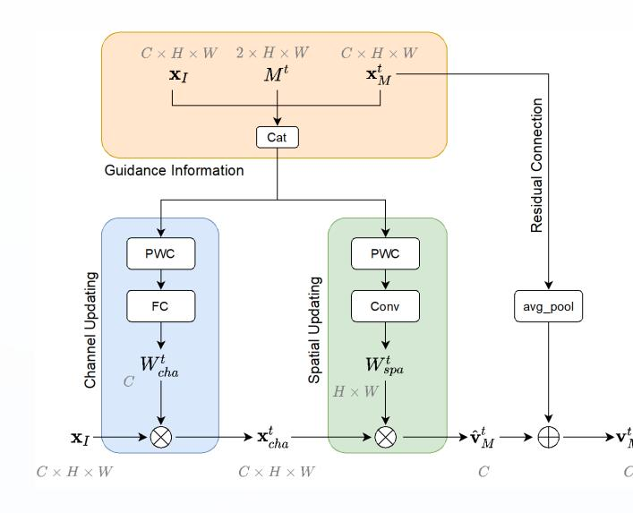
The SCCE module integrates the features of the reference I-frame when computing the features of P-frames in both channel and spatial dimen-sions. This module projects I-frames and P-frames into the same feature space.
