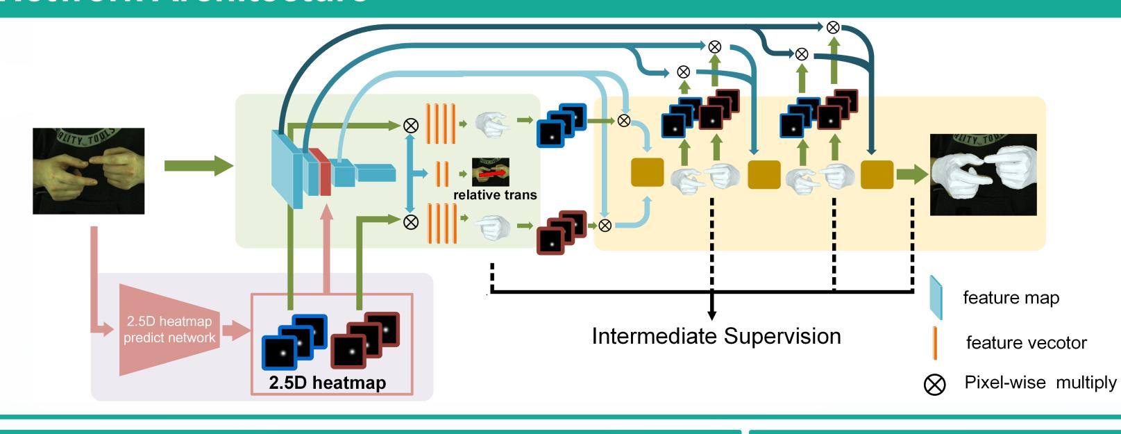
Our network first predict 2.5D heatmap for the joints of the two hands. Then use three branches to recover MANO model parameters of each hand and the relative transformation of two hands. Finally, refine the hand shape parameters jointly in a cascaded manner to respect the correlation context between the interacting hands.
